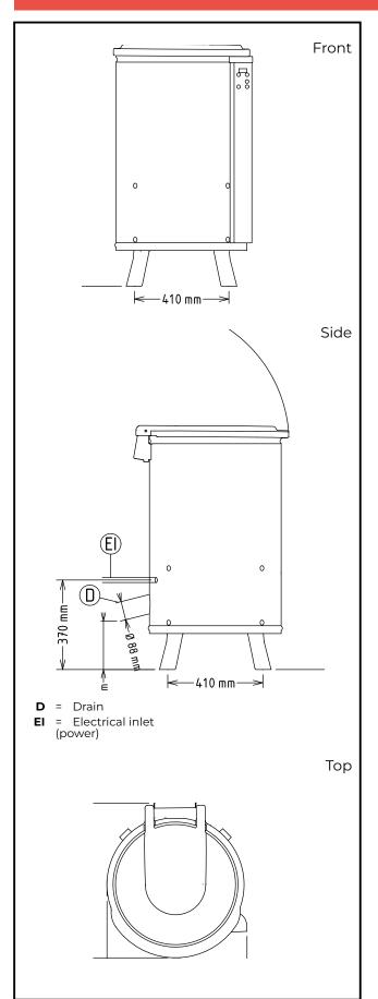
Electric Supply voltage: 220-240/380-415 V/3 ph/50 603651 (DELX65F5) Electrical power max.: 0.75 kW **Total Watts:** 0.75 kW Key Information: **Well Capacity:** 65 lt Usable well capacity: 65 lt Load per cycle - light vegetables: 18 UNITS OF LETTUCE Load per cycle - heavy vegetables: ISO 9001; ISO 14001 External dimensions, 578 mm Width: External dimensions, Depth: 639 mm External dimensions, 1005 mm **Height:**
